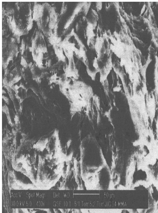
Figure 15 SEM micrograph of an Na-PCMGG-g-PMMA sample (grafting percentage = 226.47; 400 \times ).
